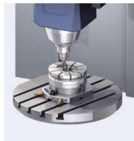
Mill off the workpiece contour
